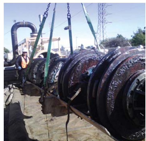
Metal bodied pigging tool following cleaning run
