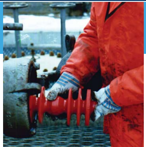
Solid cast pigging tool being positioned in a pipeline
