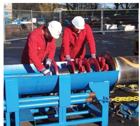
Testing of specialist pigging tool
